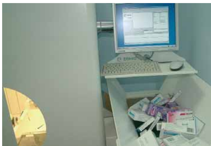
Figure 1. An automatic loader. Items for loading are tipped into a hopper, which then feeds individual packs onto a light table. An infra-red beam and a series of mirrors ensures a barcode can be detected no matter how the pack is presented.
